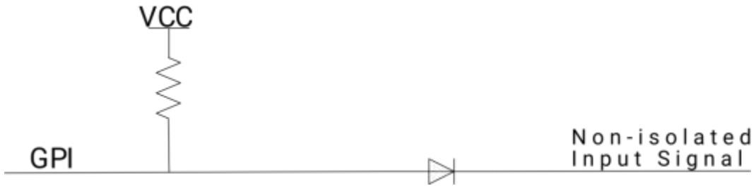
Figure 6-11 Internal Circuit of Input Signal
