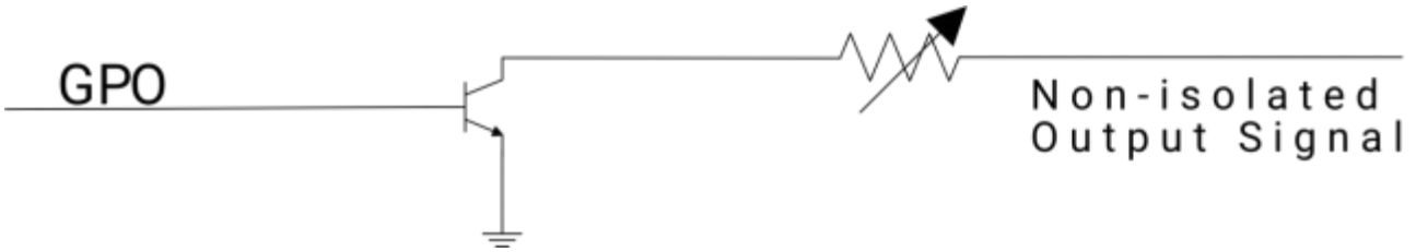
Figure 6-13 Internal Circuit of Output Signal
